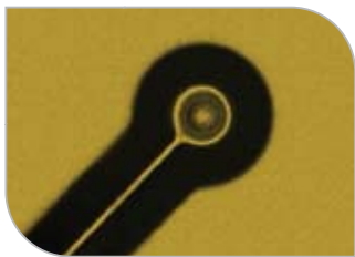
High accuracy registration results in imaging smaller annular rings
