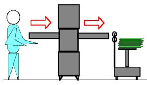
**SL13.9** is equipped with an automatic off-loader as standard. Once all the V-cuts have been made in one direction, the board is taken automatically to the rear of the machine and off-loaded. As an optional extra, a self-levelling stacker can be linked to the off-loader.
